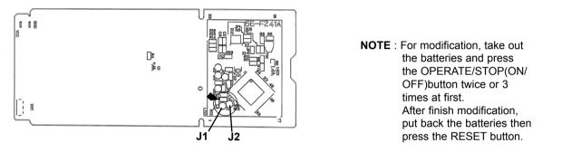
The P.C. board has the print "J1" and "J2". Solder "J1" and "J2" according to the number of indoor unit as shown in Table 1. After modification, press the RESET button.
